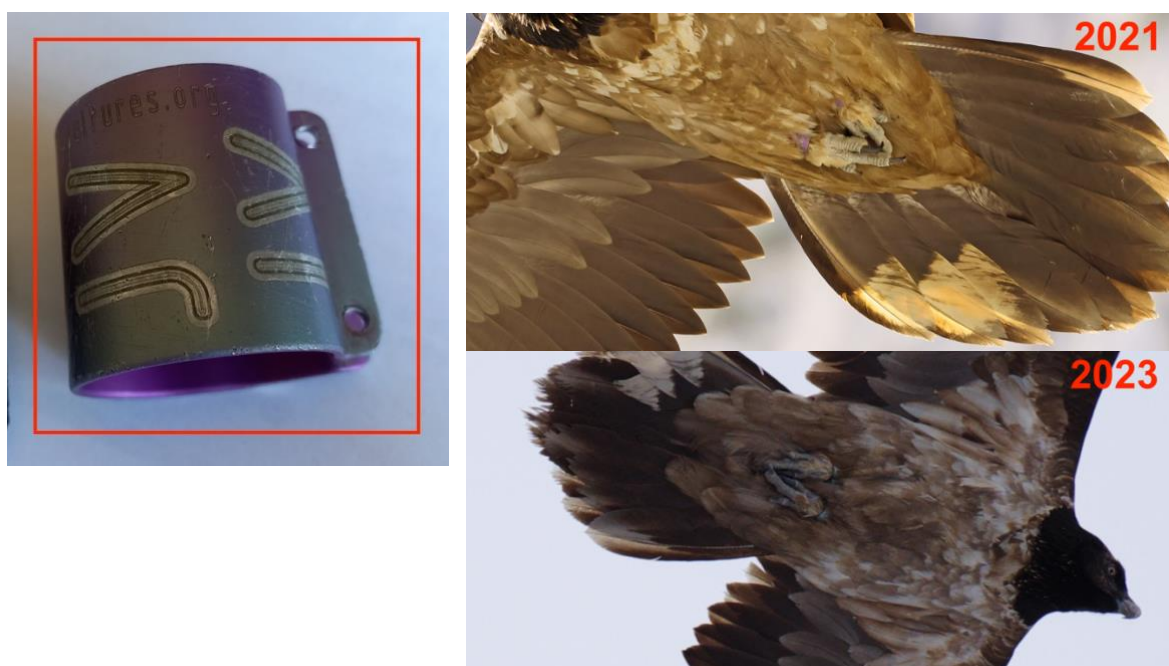
Figure 12. Anodised purple rings showed colour fading after a few months exposed to UV radiation.
