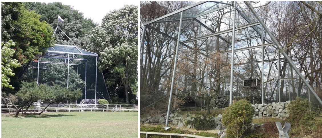
Picture 1 & 2: Potential Bearded vulture aviary surrounded with deciduous trees –assuring shadow in summer and sun in winter- and with a sloping roof, side walls, and also the ground.
