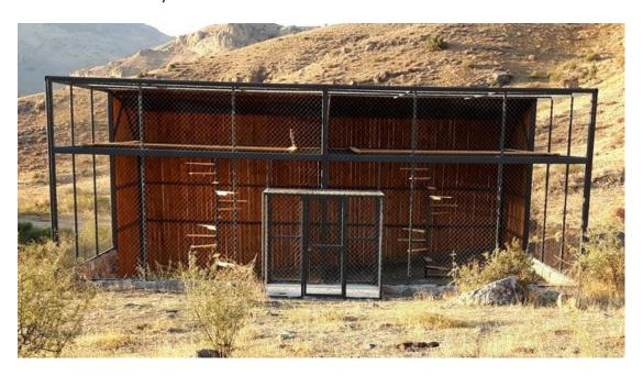
There is a continuous 4m long roof covering the almost 4m deep and 6m wide platform from both aviaries. The back of the aviary and both sides of the platforms are covered with wooden boards from the ground until the roof ensuring shedding of birds against adverse climatology. Further the parts of the aviary where neighbouring birds could have direct physical contact are closed with wood, but leaving light cracks where birds can try to break, having visual view to the neighbours.
